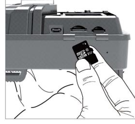
2. To remove Micro SD card, press the card inwards to release.
