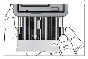
NOTE: Installing any of the 8-AA batteries in the wrong direction may cause the batteries to leak acid and could possibly explode, causing camera failure and damage to the battery compartment.
