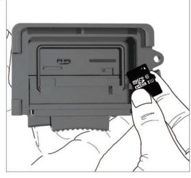
2. To remove Micro SD card, press the card inwards to release.
